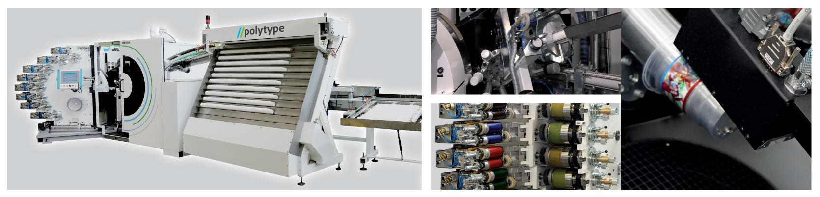
The //polytype BDM 681/682 is very user-friendly and designed for one-man operation. All main components are easily accessible and every inking unit can be swung out individually. Functions such as automatic washing and pre-inking of inking units are available to cut changeover times. All register settings can be made on the fly.
