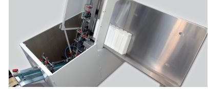
The //polytype BDM 301 is equipped with cup feeding with worm infeed. Corona pre-treatment is split between two separate stations – one for the side wall and one for the bottom. Transfer, cup positioning before and after printing, and universal cup take-off are included as standard.
