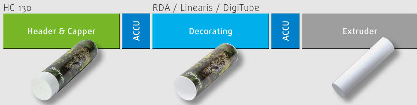
PolyLine: Sleeve in-line configuration for tube production
